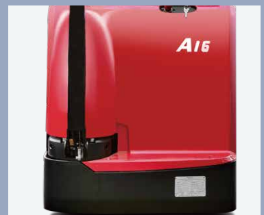
Designed to be narrow with large round corners to improve suitability for concentrated shelves and with a wedge-shape chassis to provide higher passing ability
