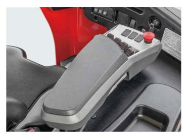
Fingertip system integrated control system, with good man-machine function
