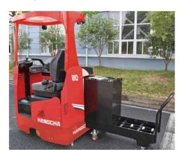
Standard configuration: Battery side roll-out + trolley(optional)
