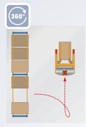
In the mode of 360-degree steering, when steering exceeds 270 degree, the reverse is switched to forward director, no reversing is required, and the truck is switched to advance automatically, no parking is required, with higher efficiency.
