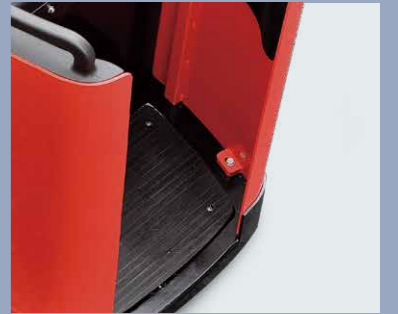
The pedal applies shock absorption design, greatly improve the operator's comfort, reduce the fatigue
