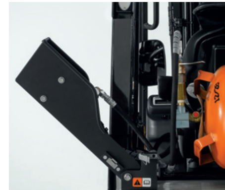
LPG reservoir tank
